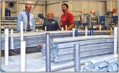
The Auburn shop fabricates 1,200 different types of stringers for 737s, ranging from 12 to 405 inches in length.
