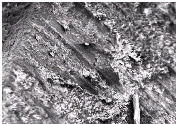
CD-4 GROOVE WALL FULL OF DIRT AFTER 100 PLAYS @ 4.5 GRAMS Figure 39
